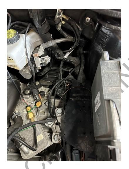
Once routed through there, pop a hole into the factory grommet with all of the other wires.....or if you are too lazy and have a DSG...you are in luck...there is an unused grommet where a clutch should be. It is perfectly fine to poke a hole and use this. Just be sure to add some form of sealant around the hole later such as 3M window weld or silicone.
