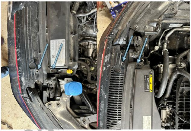
Next, remove the intake funnel, it literally just unclips and you can pull it out without much hassle. Should look like this when removed. The clips are here: (Also, pop the coolant hose off of the funnel too.)
