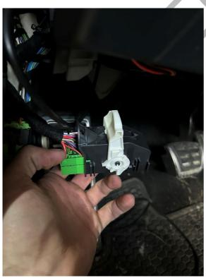
Once the plug has been removed from the housing.... Look on the plug... the pin numbers will be labeled...
