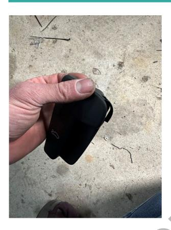
Once that is done... remove this little cover over this plastic screw.... Then remove the screw with a flathead.
